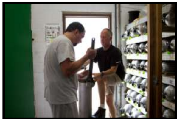
Leonard Grandbois and Scott Phillips removed the valves on the tanks to convert the old O-rings to nitrox-compatible O-rings.
